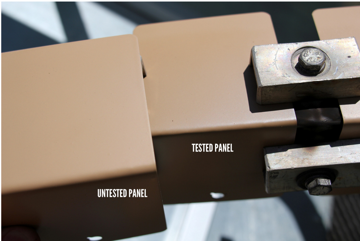
Figure 3. High Temp Brown, comparing before and after going through the exhaust system simulator.
